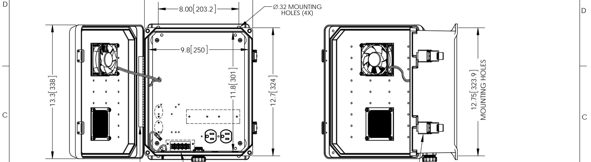
HIDDEN LINES REPRESENT COMPONENTS ON BACK OF PLATE -DO NOT DRILL-
