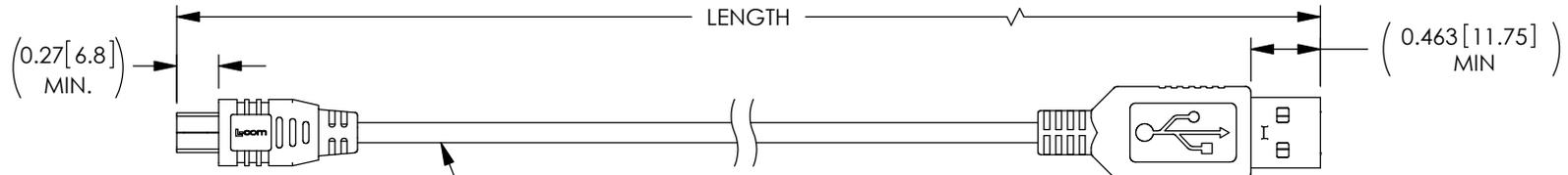
ONE 28AWG STRANDED TINNED COPPER TWISTED PAIR
