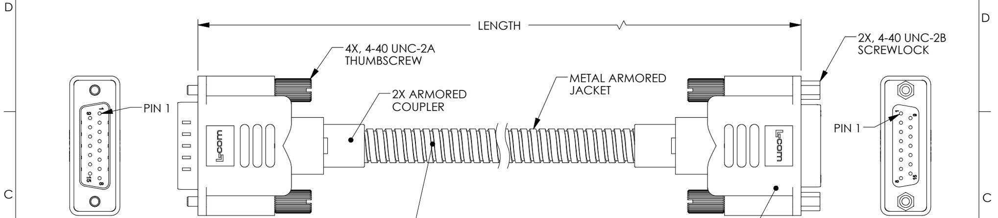
UL STYLE 2919, 15 CONDUCTOR (26AWG) CABLE WITH ALUM/POLY FOIL SHIELD AND DRAIN WIRE PLUS TINNED COPPER BRAID SHIELD. JACKET: PVC, LIGHT GRAY (PANTONE 400C)
